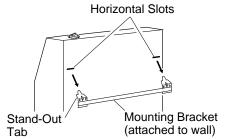
Figure 10 - Mounting Heater Onto Mounting Bracket
